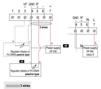
For CP112/113 – PO models and CP112/113 – PN models with 4-20 mA output – passive :
